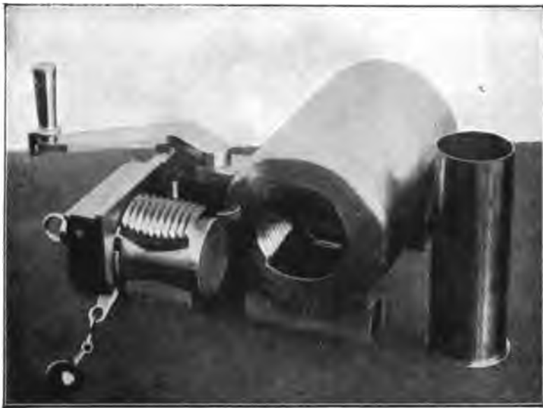
THE BREECH OF THE CREUSOT GUN
